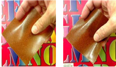
Plastics made out of Crambe seed meal (left) and B. carinata seed meal (right)
